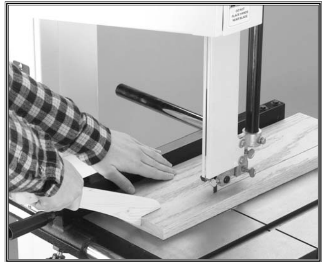
Figure 49. Ripping a board.
